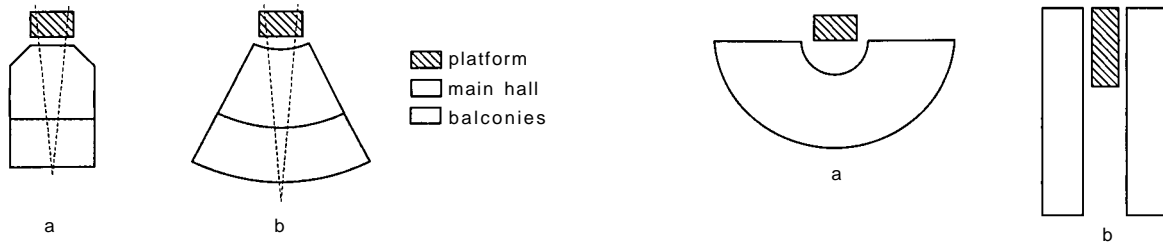
20.79 Conference hall formats for lectures requiring projection facilities: a Rectangular with or without rear balcony. b 60° fan with or without rear balcony
